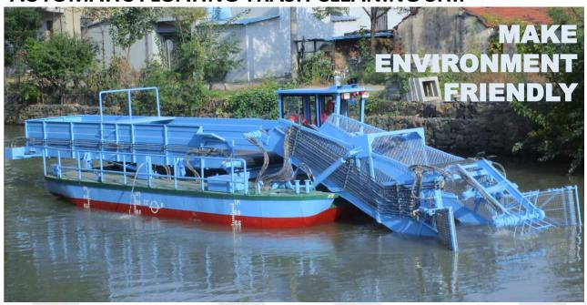
The automatic floating trash cleaning ship is an environmental protection engineering ship used to clean up the floating garbage on the water surface. It's main feature as follows:
