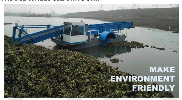
The paddle wheel cleaning ship is an environmental protection engineering ship used to clean up the floating garbage on the water surface. It's main feature as follows:
